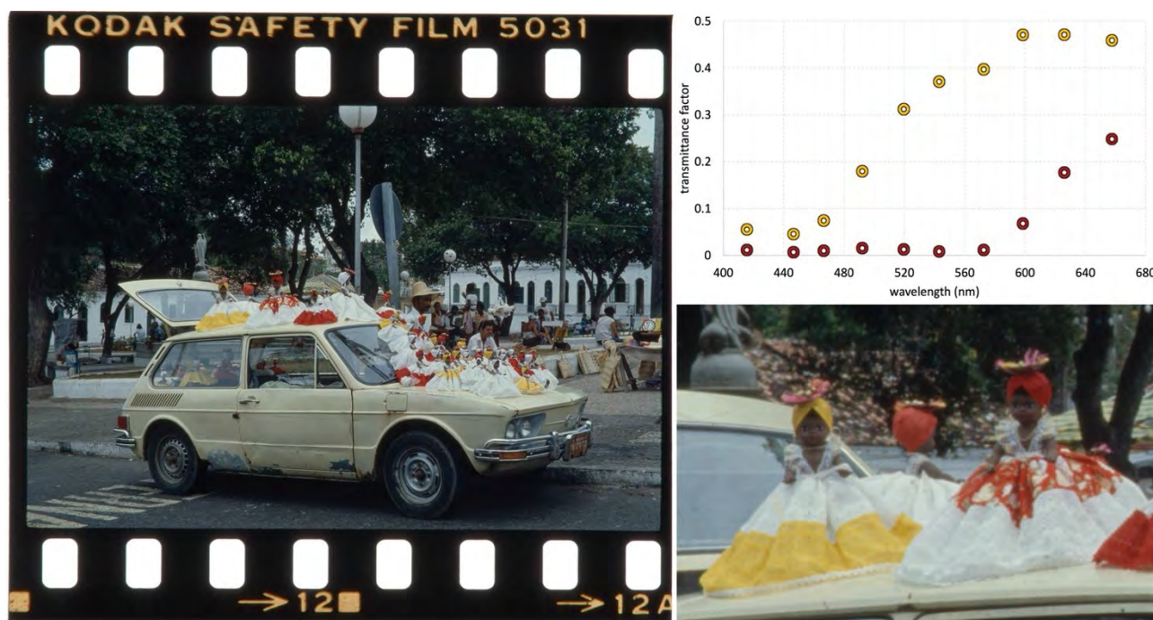
Fig. 3 - An edge-to-edge multispectral capture of a slide with the LED-based system (left). Bottom-right: Image detail of the car roof. Top-right: Transmittance values corresponding to the yellow skirt of doll on the left and to the red turban of the doll on the right. Courtesy of the Art Institute of Chicago.
