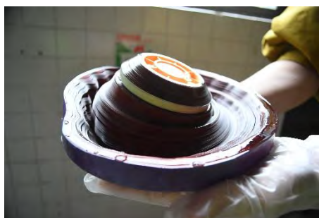
Fig. 2 - . A submerged film roll which got deformed due to the expansion of the film emulsion
