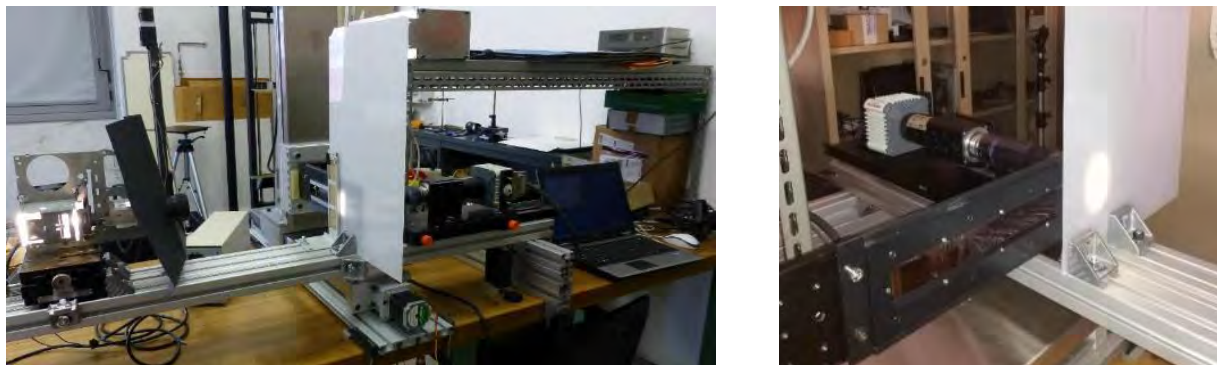
Fig. 1 - Overview of the IFAC-CNR imaging spectroscopy instrumentation set up for measurements on negative and positive 35 mm films.
