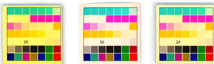
(Fig 2). Direct comparison of printing papers after hot and humid aging. Left: mounted on aluminum composite with standard adhesive; middle: printing paper not mounted, right: mounted on aluminum composite with new adhesive formulation (numbers on the samples refer to internal numbering for sample identification).
