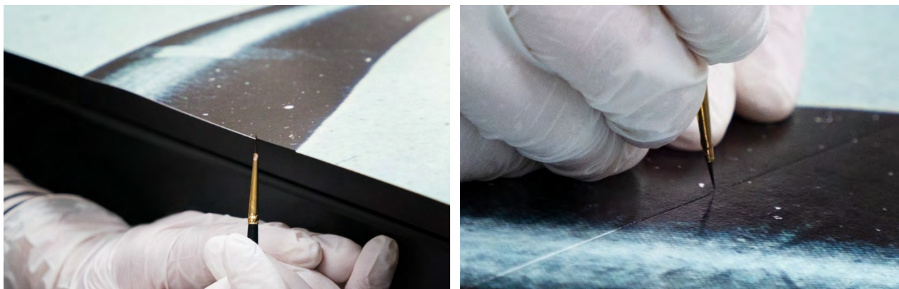
Fig. 2 – Retouching the splice seam. Left image: side view. Right image: top view.
