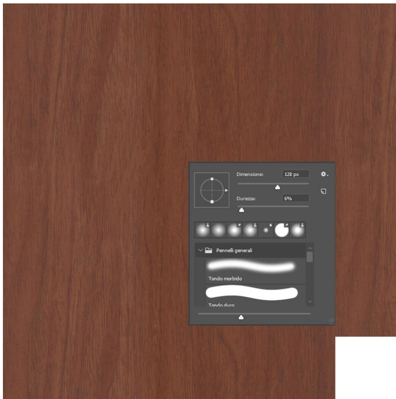
Fig 5 The texture of the same wood in fig 5 after the color calibration procedure and photo retouching to make it seamless. In the center, on the right and at the bottom, where the texture has been repeated, the discontinuities are no longer visible.
